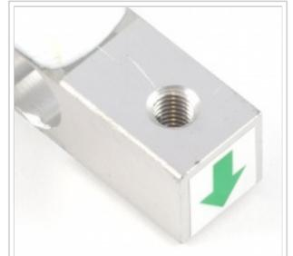
A single-point load cell. Applying force to one end creates stress in the bar, causing the strain gauge encased in the white plastic to flex.
